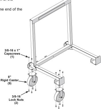
4. Attach two 8" swivel casters (10) to the other end of the chassis assembly using four 3/8-16 x 1" capscrews (1) and four 3/8-16 lock nuts (2) on each.
