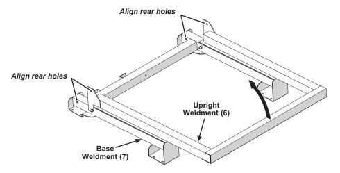
b. Secure the upright weldment (6) in place using one 3/8 x 2-1/2" snapper pin (8) through these holes on both sides.
